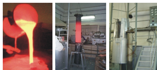
Figure 15. Molten salt (left), heated reactor vessel (center) and molten salt equipment (right)
