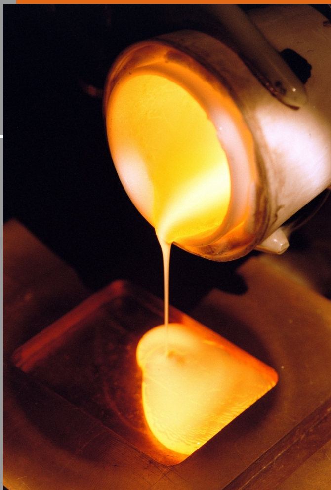
Glass matrices to contain industrial and radioactive wastes
