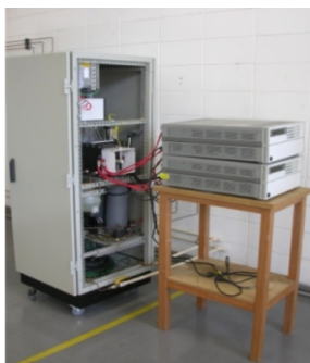
Figure 13. 1kW PEMFC system made with IPEN technology
