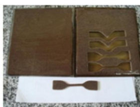
Figure 8. Gelatin/Brazil nut Shell/Nanoclay
