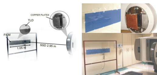
Figure 1. Experimental configuration for TSET dose distribution measurements using TLD and radiochromic films
