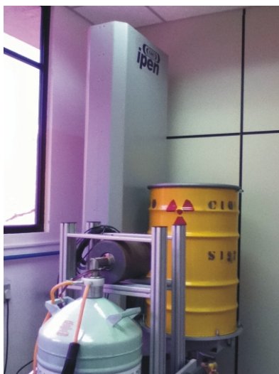
Figure 2. Automated system for isotopic characterization of radioactive waste drums
