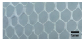
Figure 17. Sintered ceramic yttria based membrane for biogas burning
