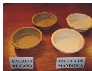
Figure 48. Foams of Starch and Sugar cane bagasse for packing application
