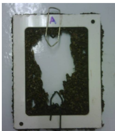
Figure 8. PVA films, prepared by casting process, were examined for biodegradation by composting over 60 days
