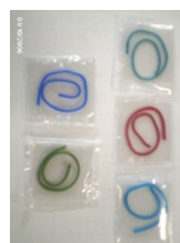
Figure 49. Silicone matrix with natural oils for repellency
