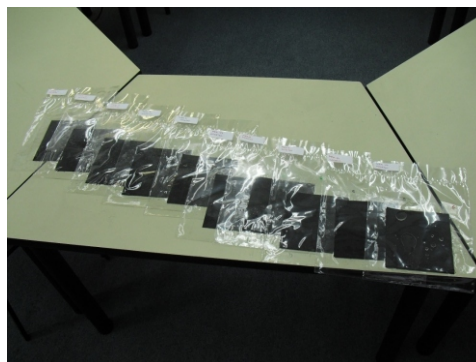
Figure 3. Membrane-Electrode-Assembly (MEA) with 250 cm 2 electrode area fabricated by sieve printing
