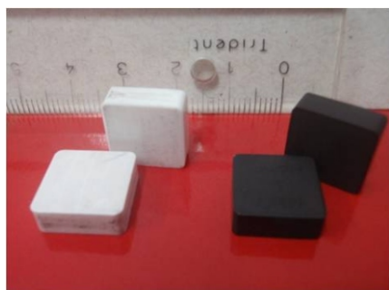
Figure 4. Ceramic cutting tool produced with alumina matrix composites
