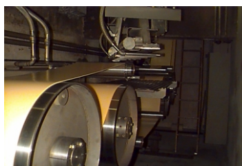
Figure 7. Low density polyethylene foam processed by ionizing radiation
